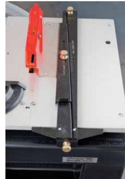
▲ This is a close-up of the upgraded T-square table saw fence with the Vernier scale. By loosening the brass knob on the top of the fence, the user can make adjustments of .005 inches by the graduated lines, and approximate close to .001 inch changes by reading between the lines.
