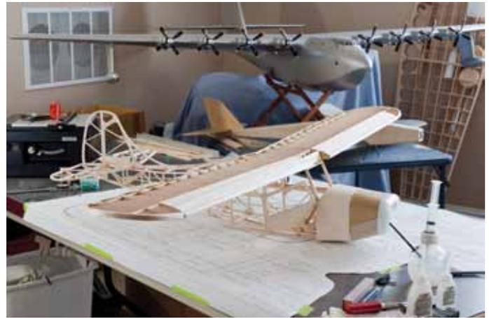
A close-up view, these magnets secure each part into place on this Aeronca Champ wing as the glue dries. The main wing spar is an "I-beam shear web" type with 1/8 in. square spruce strips on bottom, 1/16 in. balsa webs, and a (soon to be glued in) 1/8 in. spruce top strip.
