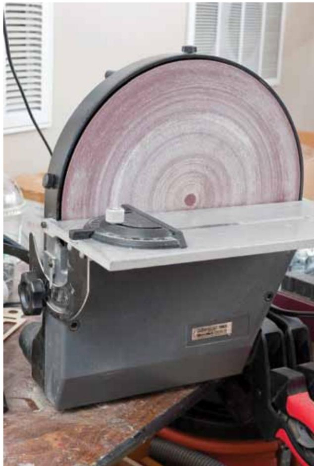
▲ This is my well-used, 10 in. Micro Mark variable speed disc sander. On the left side is the bevel adjustment for both positive and negative fence angles, and the sliding miter fence sits in a slot on the table top.
