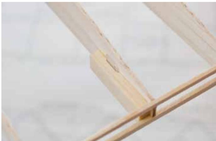
▲ The finished dado slot receives the modified nylon hinge and the hinge sits flush with the surface of the piece.
