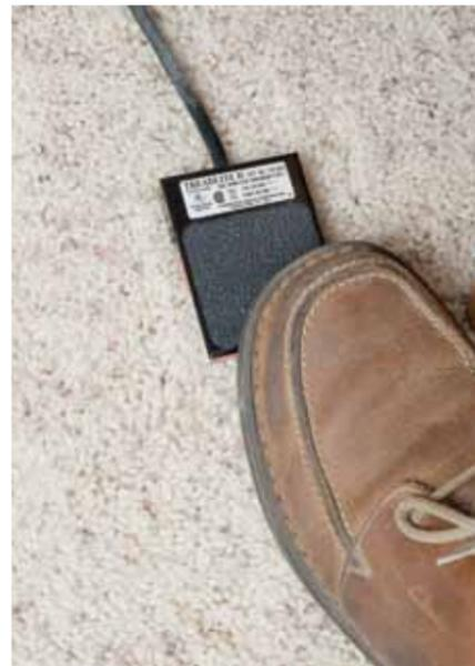
▲ The variable speed disc sander is one of the handiest tools in my workshop because of this foot pedal. By plugging in line with the 120V power cord of the sander, a slight press controls the sander for quick adjustments to sticks and parts.
