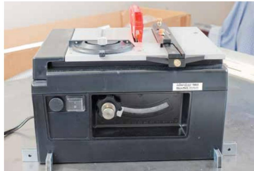
▲ The variable-speed table mini-table saw from Micro-Mark® is at home on my metal work top. The knob on the front left controls the speed of the blade and the other knob, to the right, adjusts the blade height. A larger knob, behind the height knob, adjusts the blade angle.
