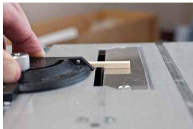
Here you can see that all of the material has been removed from the notch using back and forth motions. Note that the protective guard has been removed from this saw to show the cutting process clearly.
