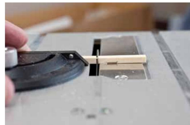
The next step is to cut the piece to length. This is easily done by setting the saw blade slightly higher than the thickness of the material being cut and passing it through on the proper side of the line. TIP: Always leave your line!
