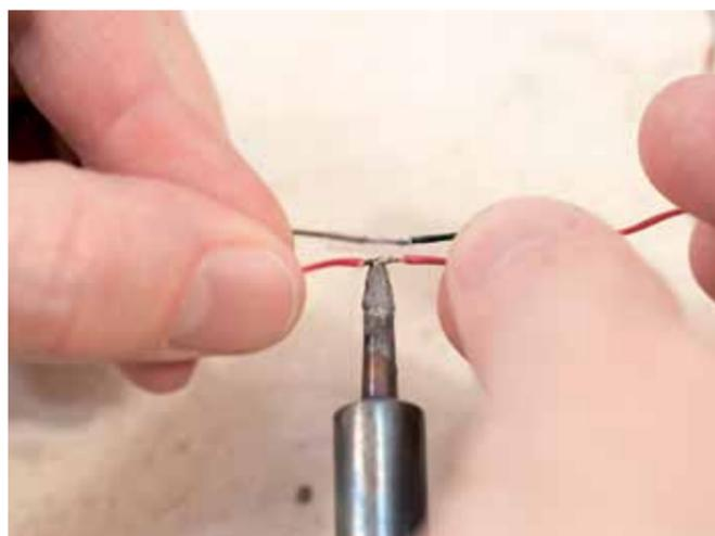
Once the two wire ends are tinned, slide a short length of heat shrink tubing over one end, making sure it's moved a safe distance away from the heat zone. Secure the soldering iron in place, then align the wire ends alongside each other, and allow the joint to meld together as it's placed on the soldering iron tip.
