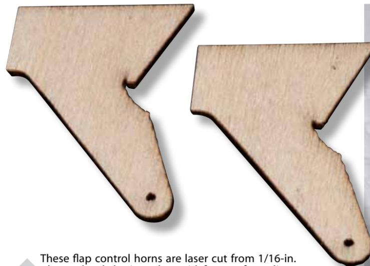
These flap control horns are laser cut from 1/16-in. plywood and glue into place with foam-safe medium CA into the user-cut slots in the flap surface.
