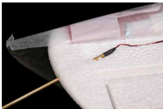
I used a piece of 5/32-in. brass tubing as effective "fish-tape" to make the tunnel and pull the light bulb and wiring through it. The 3-mm head of the navigation light fits perfectly into the brass tube, and a piece of heat-shrink tubing locks it temporarily into place.
