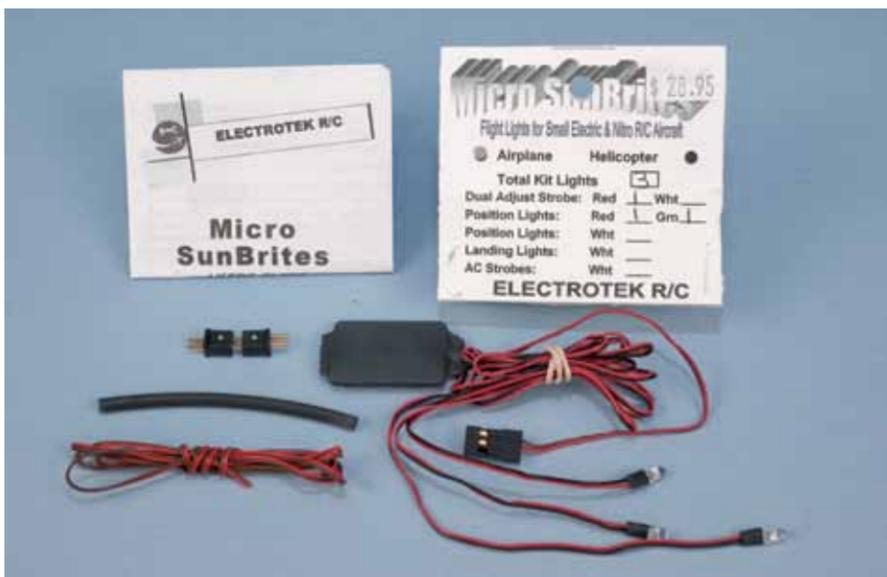
This “Micro Sun Brite” parkflyer light system is a pre-wired aircraft lighting package. The included surplus wire, shown at left, was used to lengthen the wing lights length, and the red ramping beacon was installed on the top of the fuselage, immediately forward of the fin.
