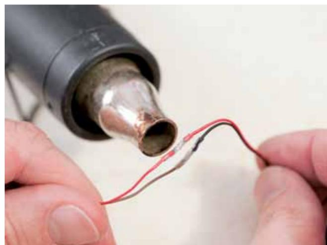
Using a pencil type heat gun with a narrow nozzle tip (available at craft stores), the clear heat shrink tubing was slid over the now cool solder joint, and shrunk into place with heat.
