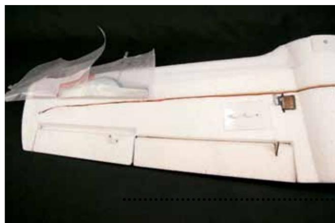
The existing stickers were heated and carefully peeled back out of the way, then safely stuck to waxed paper scraps for re-use. The wire has been installed into a small, shallow groove and made ready to cover with white vinyl tape.
