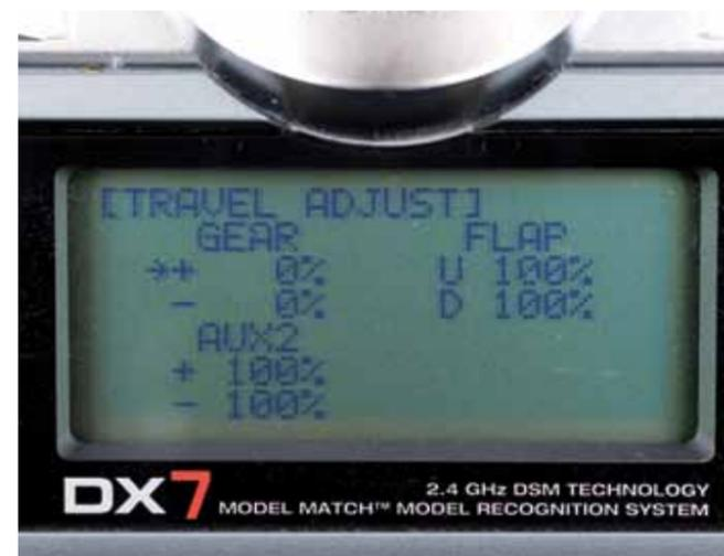
Since I plugged the flap servos into channels five and six (flaps and gear respectively), it was necessary to join them together using the programmed mix one. The user selects the flap to gear, then sets the range to plus and minus 100%.
