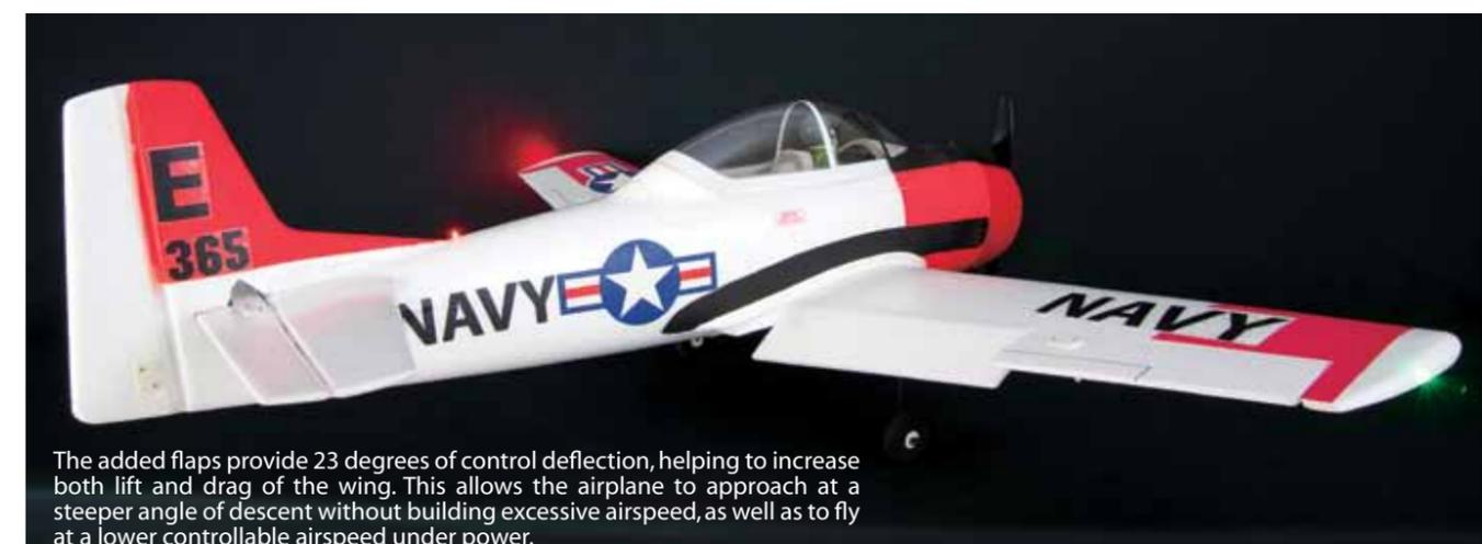
The added flaps provide 23 degrees of control deflection, helping to increase both lift and drag of the wing. This allows the airplane to approach at a steeper angle of descent without building excessive airspeed, as well as to fly at a lower controllable airspeed under power.
