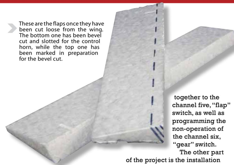
▶ These are the flaps once they have been cut loose from the wing. The bottom one has been bevel cut and slotted for the control horn, while the top one has been marked in preparation for the bevel cut.
