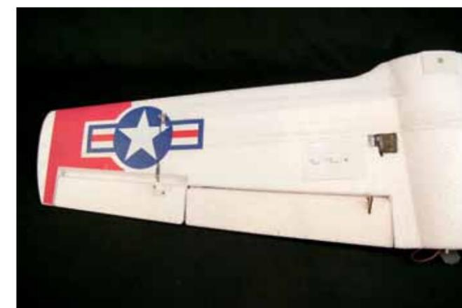
The stickers have been reinstalled, and new white vinyl tape placed, over the now-hidden wire installation to the navigation light in the wingtip.
