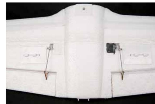
Dubro Mini E-Z connectors and micro links connect the .047 music wire to the servo and flap control arms. The servo on the left has been covered with the white vinyl tape, and is nearly hidden from view.
