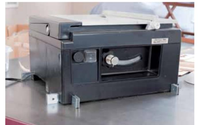
▲ Latch magnets can be used to keep things from sliding on the worktop. Here they are placed at each corner of the Micro-Mark table saw to secure it in place.
