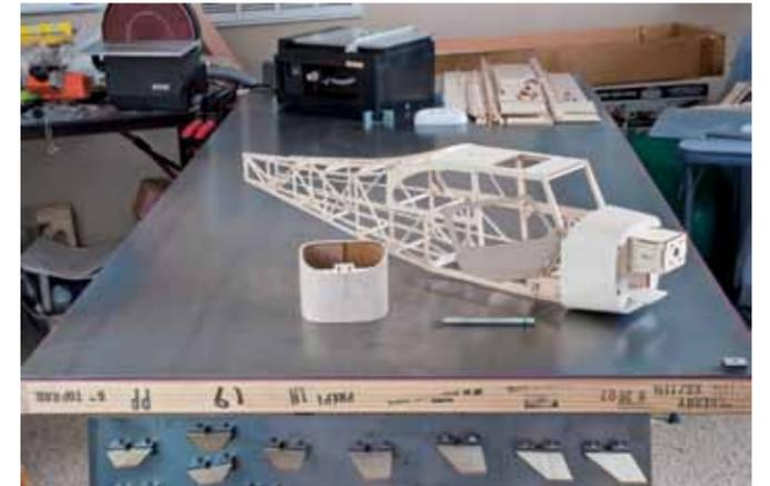
▲ The table top is a generous, 3 by 7 foot flat surface, shown here with the Aeronca Champ fuselage and cowl. The trusty 10" disk sander and table saw stand ready in the background, while spare jigs await use in the foreground on a scrap piece of steel beneath the table.
