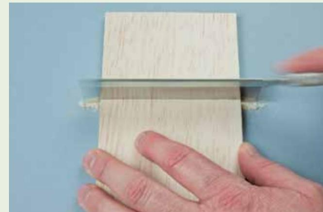
Remove the protractor after marking the cut, and then cut through the plank while ensuring the blade is kept plumb.
