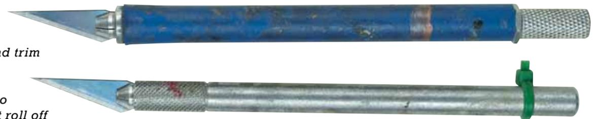
Two versions of hobby knives, both with sharp #11 XACTO® blades installed. The blue “soft grip” version has a hex nut on the end which prevents table roll-off, while the aluminum handled version has a zip-tie attached for safety.
