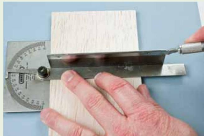
On thicker sheets of balsa, start with a razor saw against the edge, being careful to not hit the metal protractor head, and pull the blade away from the piece to mark the line.
