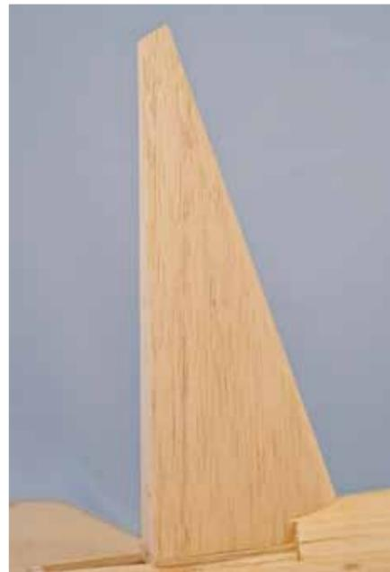
This flat fuselage side of a simple model was cut from B-grain balsa and has a strong resistance to both splitting and bending. This will prevent possible breaking of the sides should it be gripped between inner supports.
