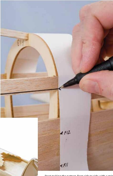
Start making the pattern, from side to side, with a strip of paper wrapped on top of the first former. The length is marked on the paper strip and labeled as such, and the process is repeated for the rest of the formers.
