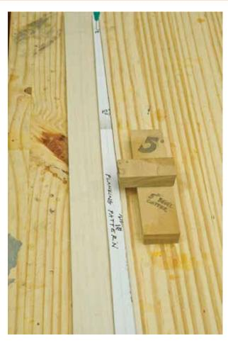
The pattern has been glued to a piece of 1/32-in. plywood which is shown pinned down to a piece of 3/16-in. med-soft balsa. Using a homemade, bevel, cutting fixture, the blade follows along the plywood edge to cut at an outward angle, then repeated on the opposite edge in the same way.
