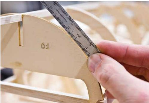
Check to see how the calculated plank width will look with a ruler placed on the former, allowing no more than 1/32-in. of gap from the ruler to the former on each side. The best plank width is likely to be from 1/4- to 5/8-in. for most of our models.
