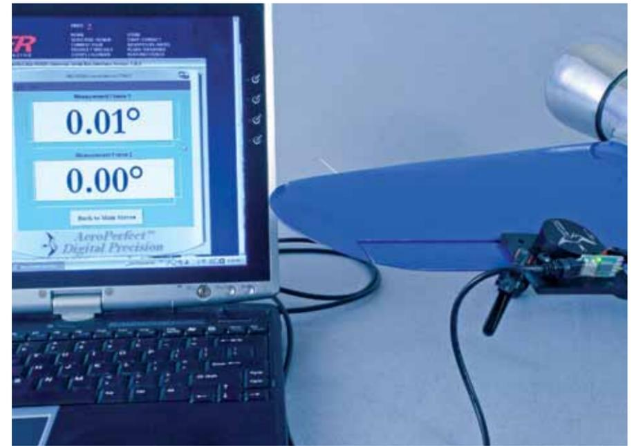
to a computer to measure, set and verify angles of surface throws, wing and stabilizer incidences and decalage (angle formed of wing incidence versus stabilizer incidence) of your airplane. The unit consists of a small measuring head that measures only 2 x 3 x 0.75 in. Tall, which connects to your laptop computer with an included 6-ft USB cable. The unit does not require any batteries and draws the necessary power from
