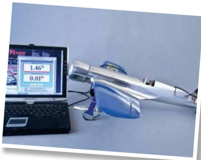
After establishing a neutral reference point, the measuring head is placed upon the flat plate stabilizer of this 32-in. wingspan Hughes racer and the incidence shown on the screen is 1.46 degrees
