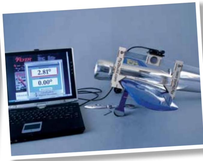
The wing incidence is measured next and the resulting angle is 2.81 degrees of positive incidence relative to the neutral reference point.
